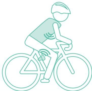
The system uses an algorithm and two sensors which are able to distinguish cyclists' common movements in an accident. The CDU sensor (crash detection unit), located inside the vest, analyzes cyclists' motion in real time and the SDU saddle sensor detects the shock. When an abnormal move or a shock is detected both sensors communicate with each other and analyze the situation.
