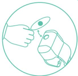
**3. Place the magnet on the saddle sensor** over the round sign. Please note that you only have 30 seconds to effect this procedure.
