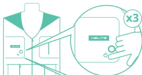
**1. Switch ON** the vest by pressing quickly 3 times the button
